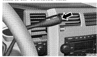
When driving in hilly areas, towing a trailer, carrying a heavy load, etc., and frequent transmission shifting occurs, press the "TOW/HAUL" button. This will improve
